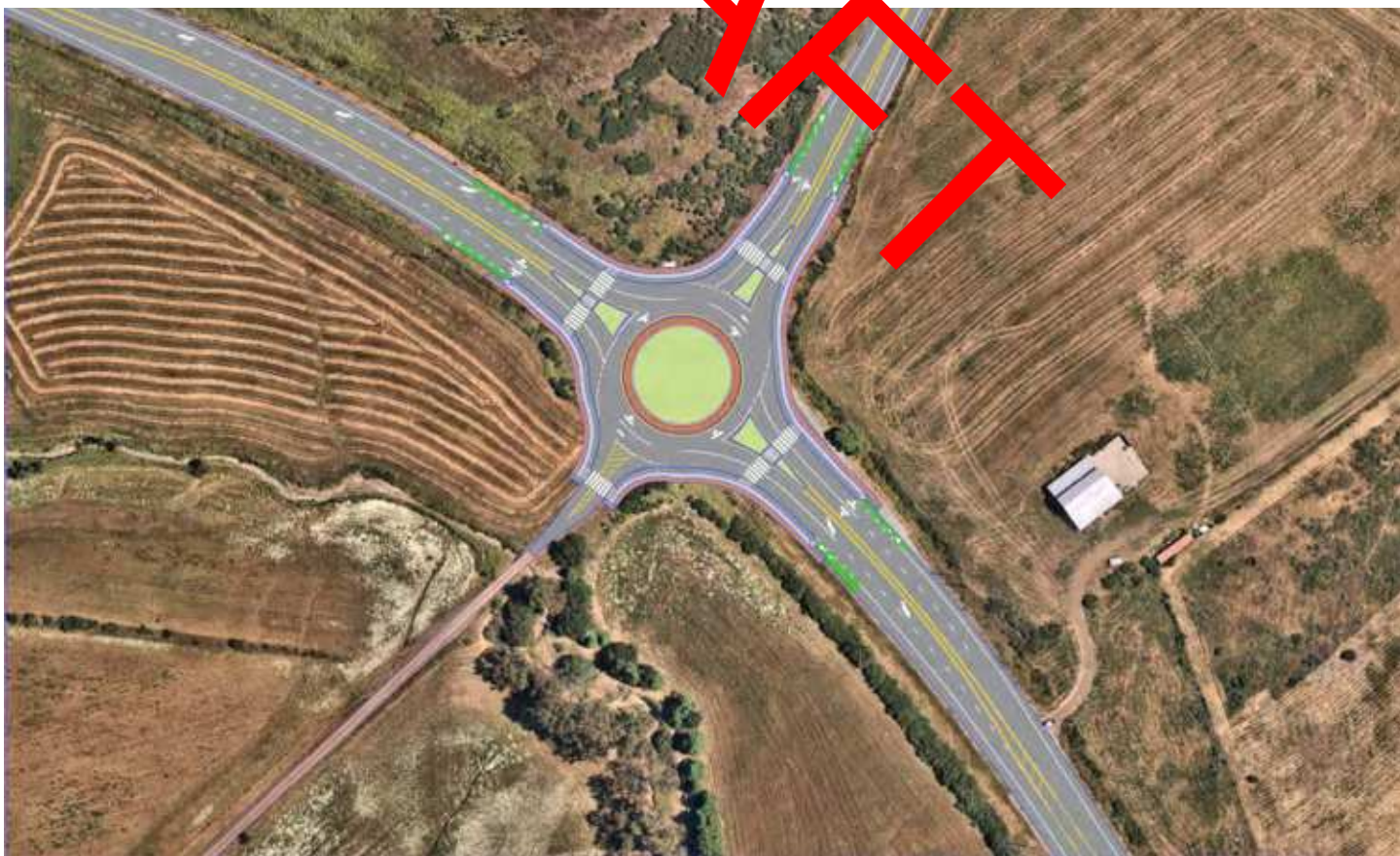
Exhibit 56. Proposed single lane roundabout with right-turn lane
